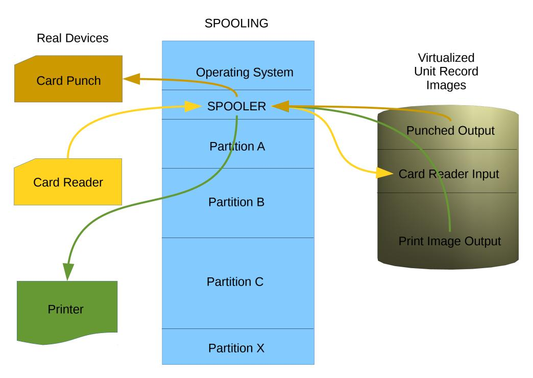
All partitions simultaneously perform I/O to the virtual unit record devices
