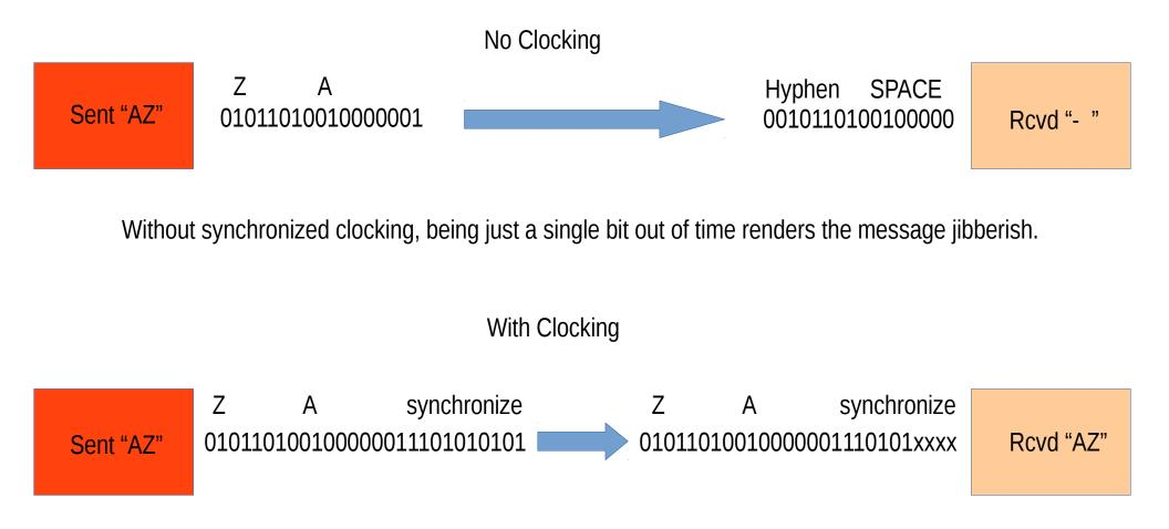
A set of characters to be transmitted is prepended with a synchronization sequence that the receiver will recognize as a request from the sender to synchronize the ticks of their clocks.
